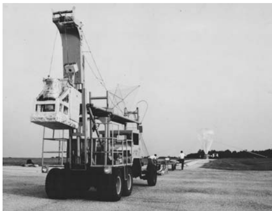
Fig. 4.47. The launch layout for the first flight of the new payload. The package has been lifted by the launch vehicle ASCEND II. The payout reel with the 700 m of line is on the cart between the launch vehicle and the balloon. At the time when the picture was taken the top of the balloon was being filled with helium. The lower part of the balloon is lying on a tarpaulin between the cart and the clamp that is holding the balloon down. Although they are not visible, there are separate parachutes in the flight train for the reel and the payload. Once the balloon is released the launch crew member with his foot on the cart will follow the path of the balloon as it lifts the reel off the cart. ASCEND II will chase the balloon around the field until it is a little down wind of the vehicle and then release the payload. If the launch master has been successful, the payload will go forward and upward rather than backward and hit the vehicle. The launch ballet and the balloon dynamics are lovely to watch and much quieter than a spacecraft launch.
