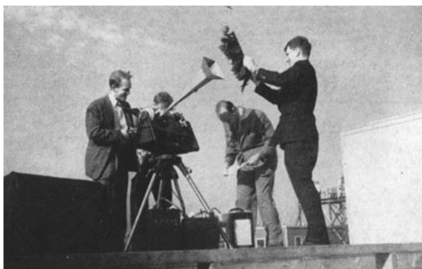
Fig. 3.2. A Dicke microwave radiometer. From the left E. Beringer, R. Kyhl, A. Vance, and R. Dicke. Dicke is holding in front of the horn antenna a “shaggy dog,” a good approximation to a source of blackbody radiation at room temperature. (From Five Years at the Radiation Laboratory , MIT, 1946.)
