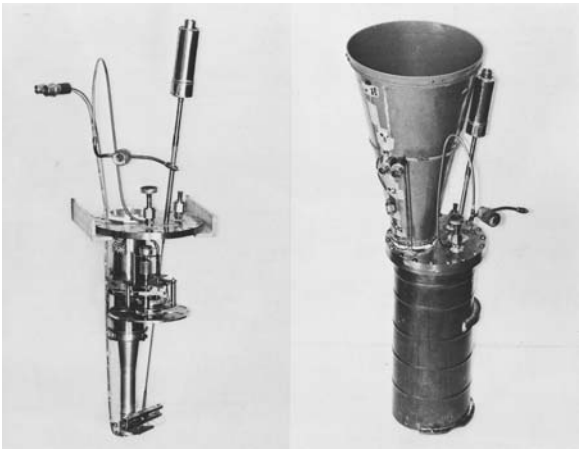
Fig. 4.44. Left: photograph of the radiometer showing the filter transport and chopper; right: the sealed copper can with the radiometer installed.
